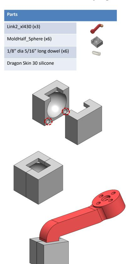
Insert the Ø1/8" dowel pins in the holes marked by the dotted red circles on *one* of the MoldHalf\_Sphere parts. These pins will be used to align the two halves of each mold. Depending on the print tolerances, the holes for the dowel pins may have to be reamed to be able to press fit them in. The holes on the other MoldHalf part without the dowel pins can also be drilled to provide a clearance fit for the dowel pins.
